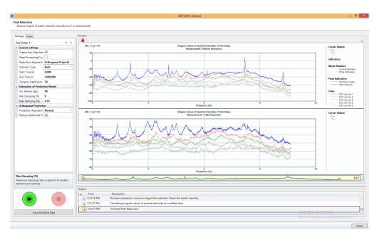
Figure 7: Removal of harmonics at 2.05Hz, 4.1Hz, 6.15Hz, 8.2Hz and 10.2Hz.
