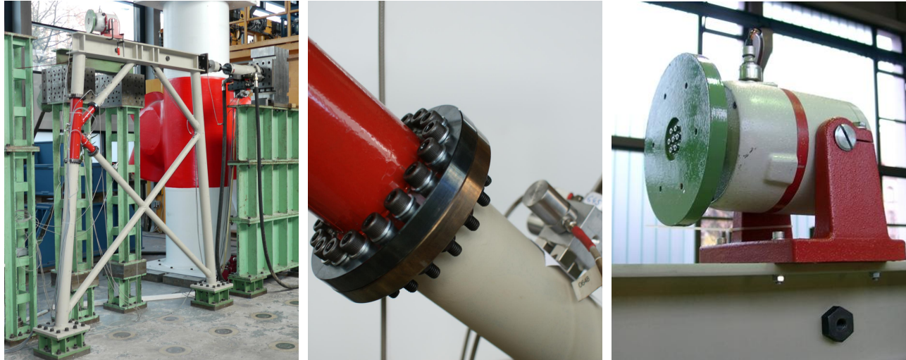
Figure 3: Test stand for proof testing of damage identification algorithms; left: laboratory structure, middle: flange connection for damage modeling, right: electrodynamic shaker for excitation
