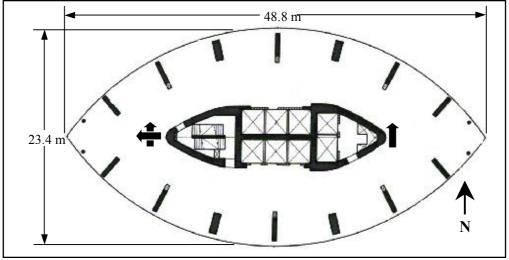
Figure 2. Typical floor plan and sensor location.
