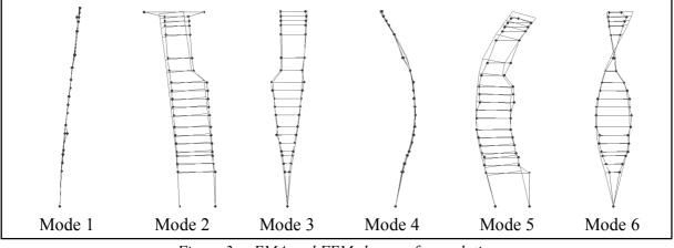
Figure 3. EMA and FEM shapes after updating.
